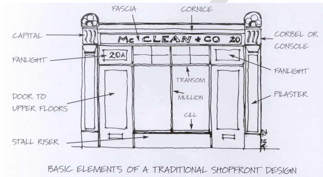
Figure 7: Basic elements of a traditional shopfront
